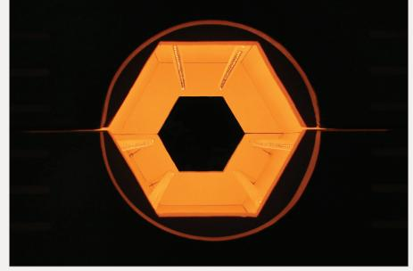
The Thermoclam 100 in use, showing the Short Wave Quartz Halogen tubes.
