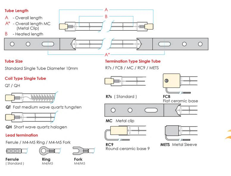
While quartz tungsten and quartz halogen tubes can be supplied individually, we also manufacture our own combined array system known as a FastIR.
