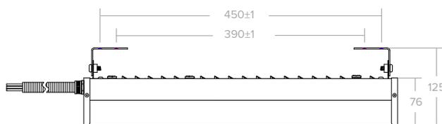
Side view with mounting brackets assembled
