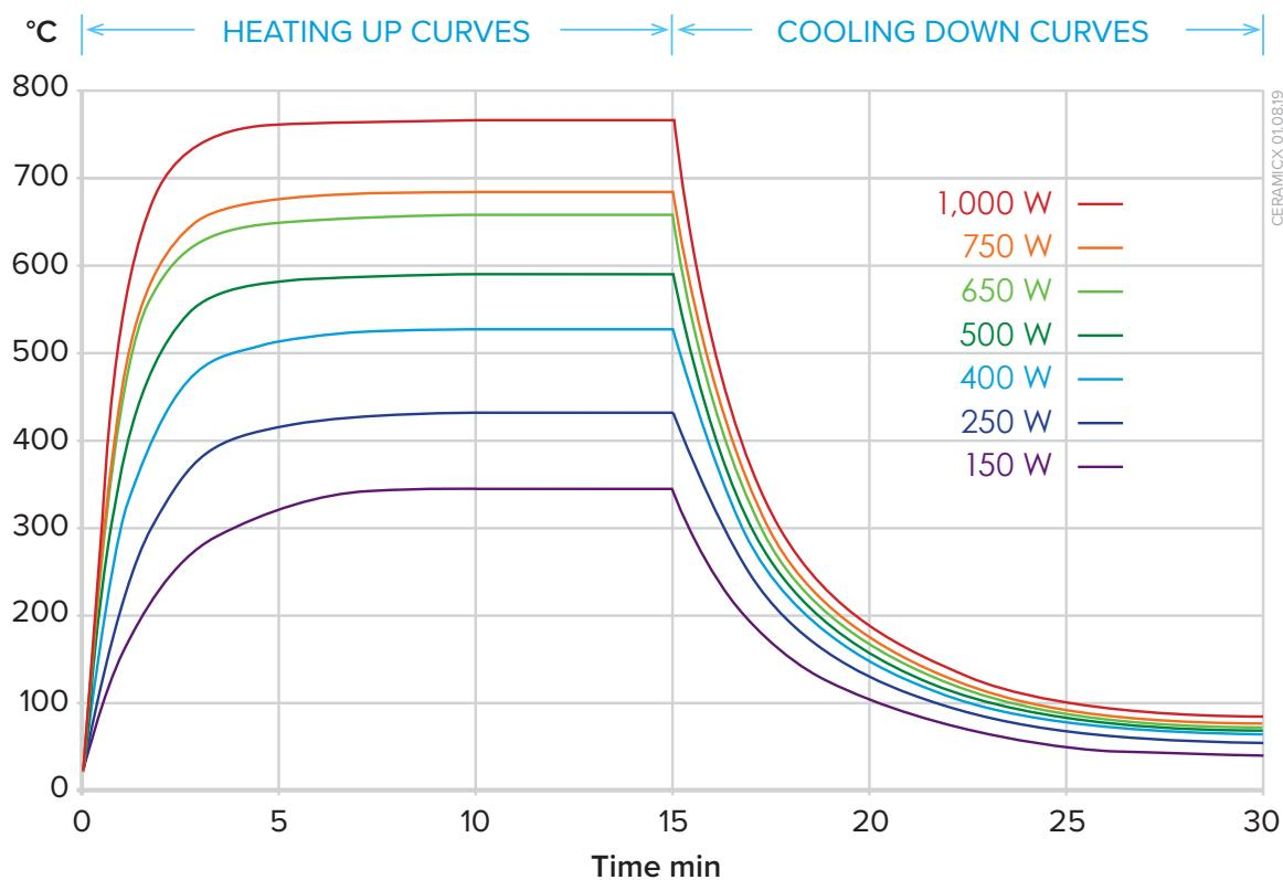
**PFQE-L TcK** Heat up and cool down curves showing average surface temperature measured with a thermal imaging camera set to an emissivity of 0.7
