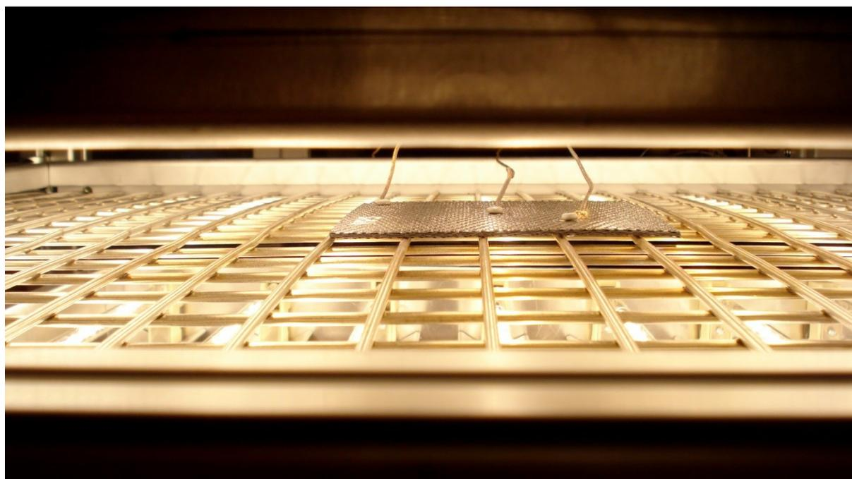
Figure 1: Sample of material between two FastIR heaters with QHL elements
