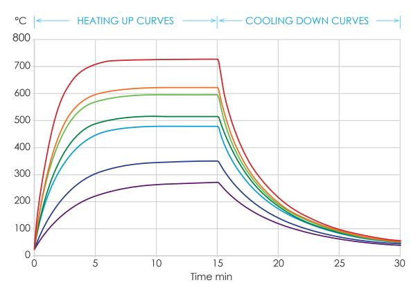
**FTE** Heat up and cool down curves showing average surface temperature measured with a thermal imaging camera set to an emissivity of 0.95 ( *element mounted in a polished aluminium clad steel reflector* )
