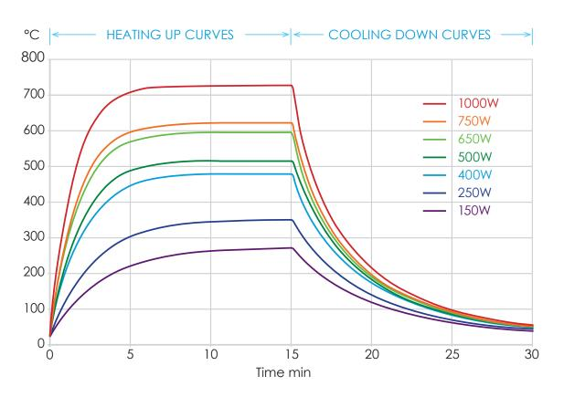
**FTE TcK** Heat up and cool down curves showing average surface temperature measured with a thermal imaging camera set to an emissivity of 0.95 ( *element mounted in a polished aluminium clad steel reflector* )
