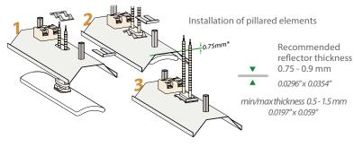
Recommended Slot hole size 42 x 15 mm 1.6535"x 0.5905"
