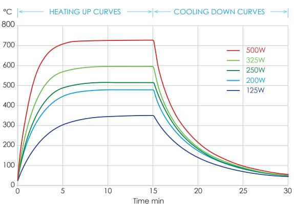
**HTE TcK** Heat up and cool down curves showing average surface temperature measured with a thermal imaging camera set to an emissivity of 0.95 ( *element mounted in a polished aluminium clad steel reflector* )
