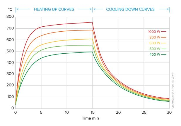
**FFEH** Heat up and cool down curves showing average surface temperature measured with a thermal imaging camera set to an emissivity of 0.95 ( *element mounted in a polished aluminium clad steel reflector* )
