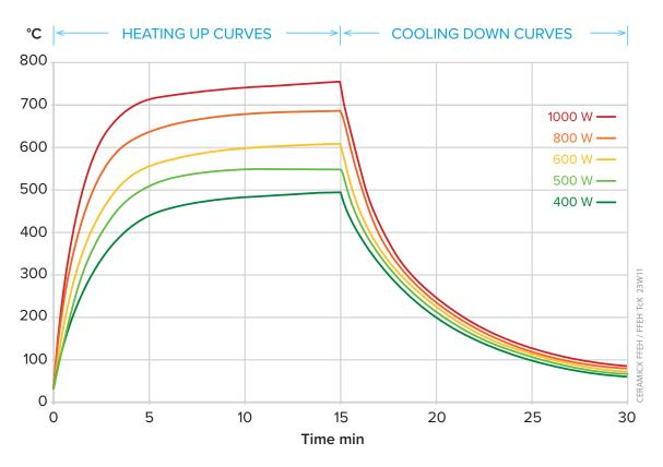
**FFEH** TcK Heat up and cool down curves showing average surface temperature measured with a thermal imaging camera set to an emissivity of 0.95 ( *element mounted in a polished aluminium clad steel reflector* )
