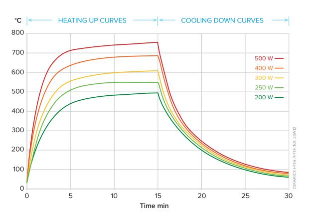
**HFEH** Heat up and cool down curves showing average surface temperature measured with a thermal imaging camera set to an emissivity of 0.95 ( *element mounted in a polished aluminium clad steel reflector* )
