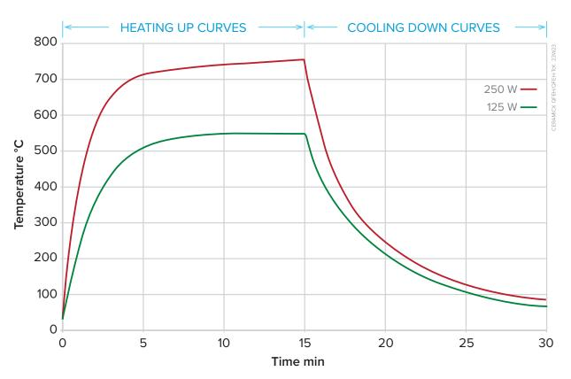
**QFEH** Heat up and cool down curves showing average surface temperature measured with a thermal imaging camera set to an emissivity of 0.95 ( *element mounted in a polished aluminium clad steel reflector* )
