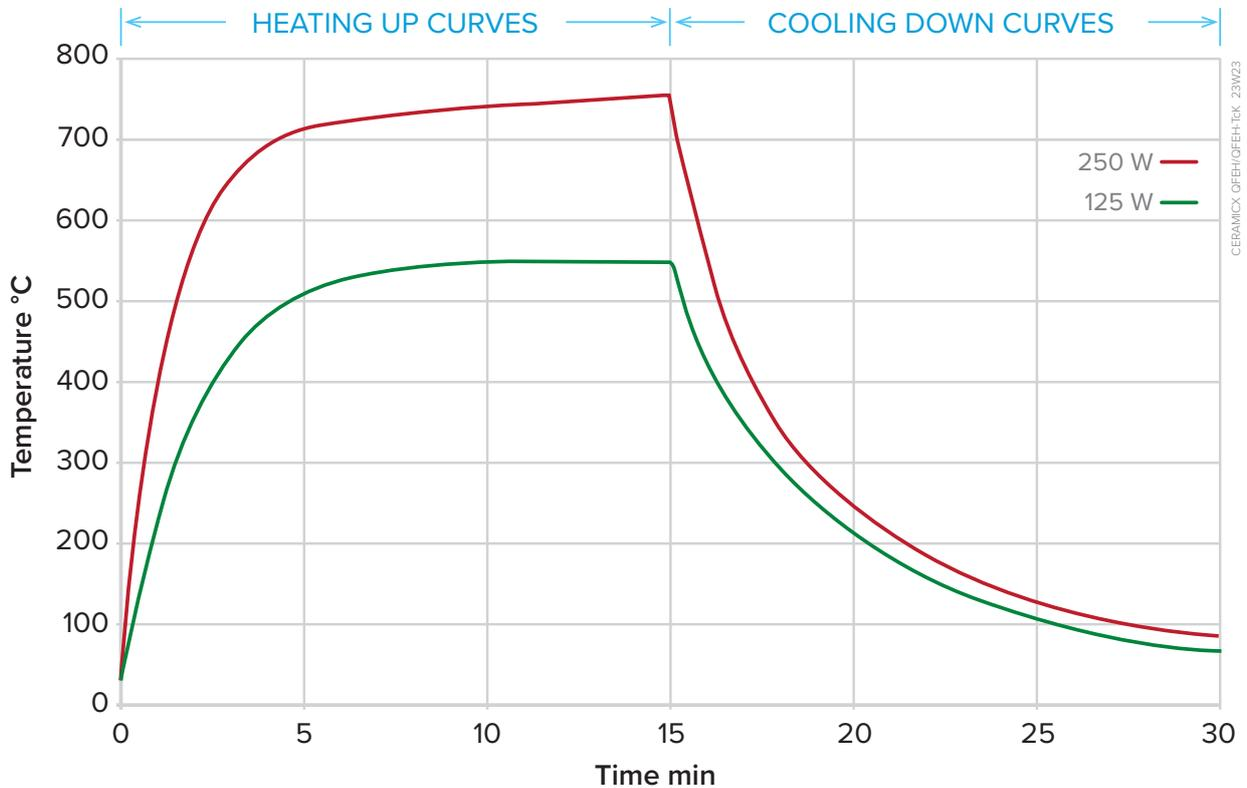
**HFEH - TcK** Heat up and cool down curves showing average surface temperature measured with a thermal imaging camera set to an emissivity of 0.95 (element mounted in a polished aluminium clad steel reflector)
