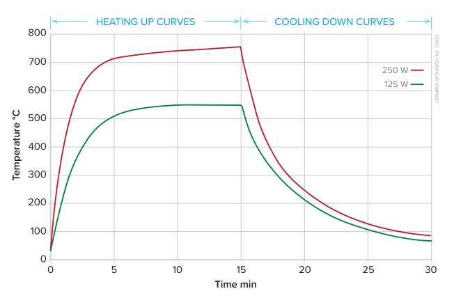
QFEH - TcK Heat up and cool down curves showing average surface temperature measured with a thermal imaging camera set to an emissivity of 0.95 (element mounted in a polished aluminium clad steel reflector)
