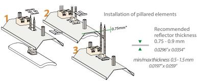
Recommended Slot hole size 42 x 15 mm
