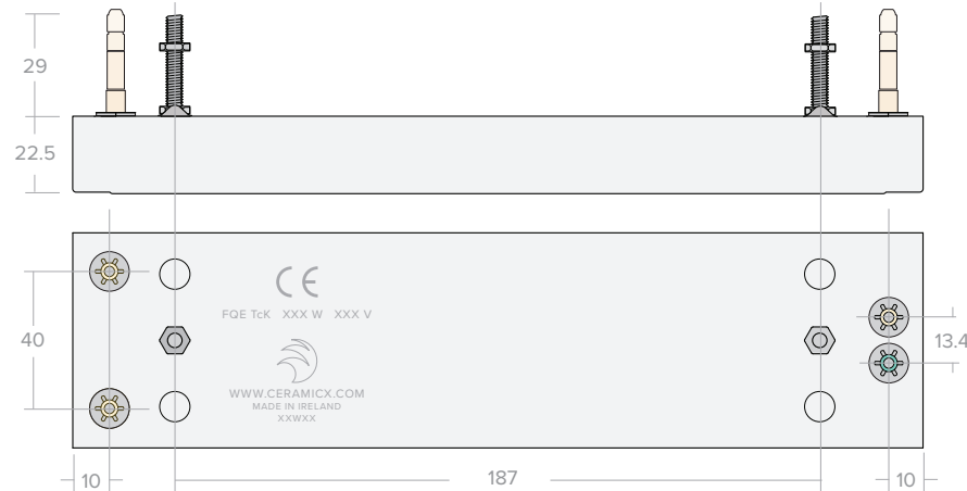
THERMOCOUPLE POSITION FOR FQE ELEMENTS HIGHER THAN 500W
