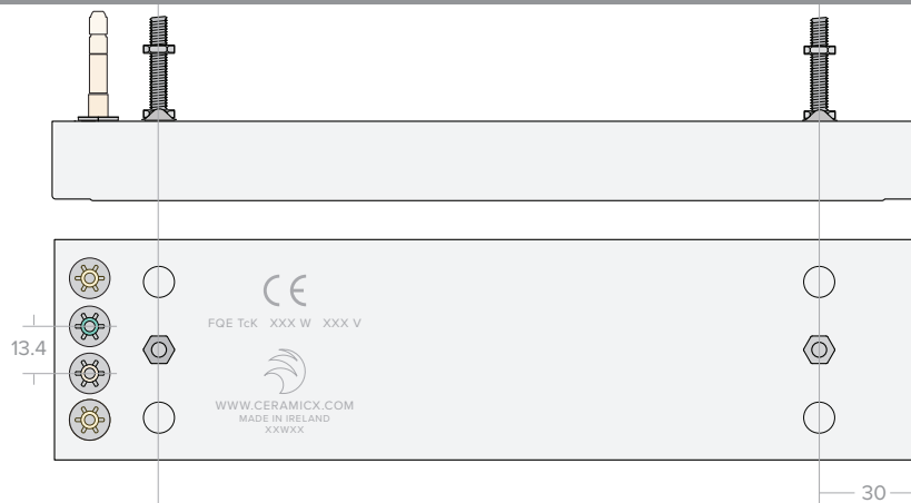
THERMOCOUPLE POSITION FOR FQE ELEMENTS HIGHER THAN 500W
