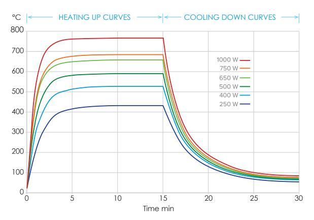
**SQE** Heat up and cool down curves showing average surface temperature measured with a thermal imaging camera set to an emissivity of 0.7
