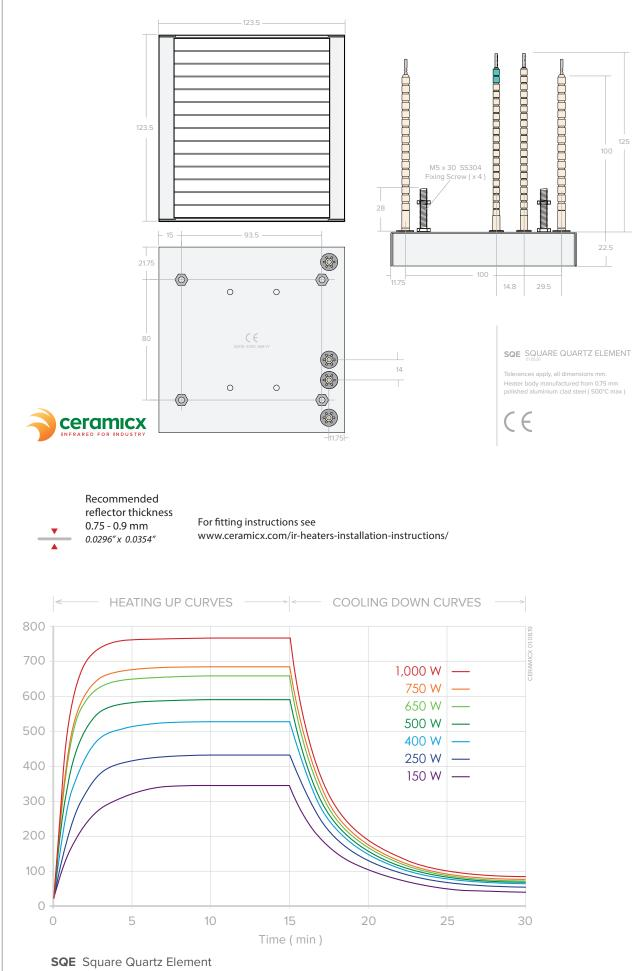
Heating up and cooling down curves showing average surface temperature taken with an infrared thermometer set at an emissivity of 0.7
