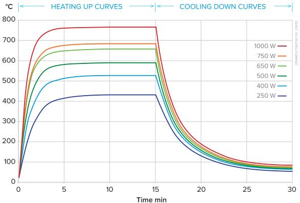
**PFQE TcK** Heat up and cool down curves showing average surface temperature measured with a thermal imaging camera set to an emissivity of 0.7
