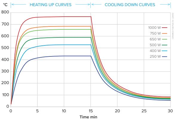
**PFQE TcK** Heat up and cool down curves showing average surface temperature measured with a thermal imaging camera set to an emissivity of 0.7
