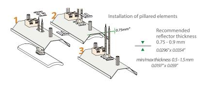
Recommended Slot hole size 42 x 15 mm 1.6535"x 0.5905"
