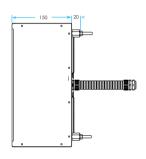
4 x Aluminium stand off with M6 threaded screw with fixing nut.
