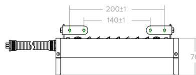
Side view with mounting brackets assembled
