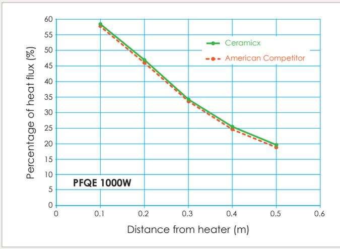
From an IR perspective alone the Ceramicx element could provide a significant cost saving. At an energy rate of \$0.10 per kW hour, and an expected lifetime of around 20,000 hours, switching to the Ceramicx FFEH could save up to \$58 per element replaced. In a platen with 100 elements, this could mean a saving of \$5800 over its operating lifetime.
