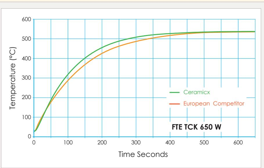
Surface temperature measured by type K thermocouple bonded to central rib at the same location on both elements under test
