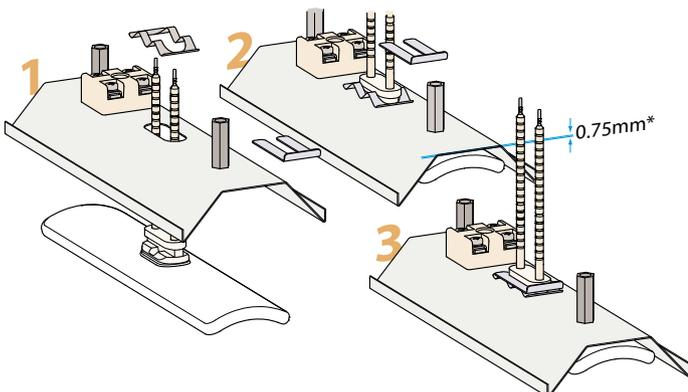
Recommended reflector thickness 0.75 - 0.9mm
