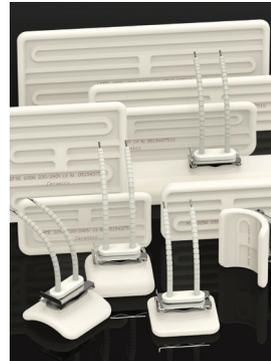
The cover shows the recent developments in our ceramic element range, the rectangular section running across the ribs brings the location of the thermocouple closer to the surface of the element, while maintaining its interaction with the resistance coil.
