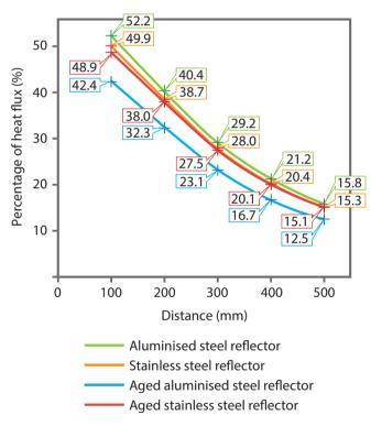
For higher temperature applications, where aluminium oxidation is likely to occur, stainless steel was found to be a better choice as the material leads to a greater proportion of radiative energy that is directed towards the target material.
