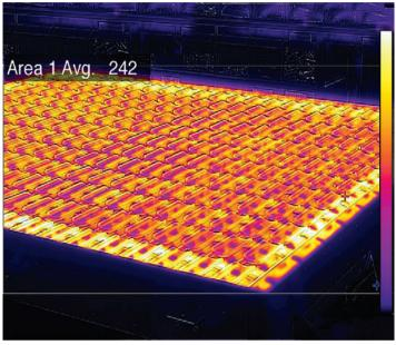
Infrared image of ceramic thermoforming platen under testing (photo -Gethyn Morgan, Green Engineering)
