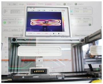
FTE ceramic element under test on our semi automated validation equipment
