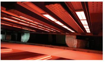
Deployment of Ceramicx 245 x 60mm IR elements succeeds in supplying a very uniform process heat for the film production.
