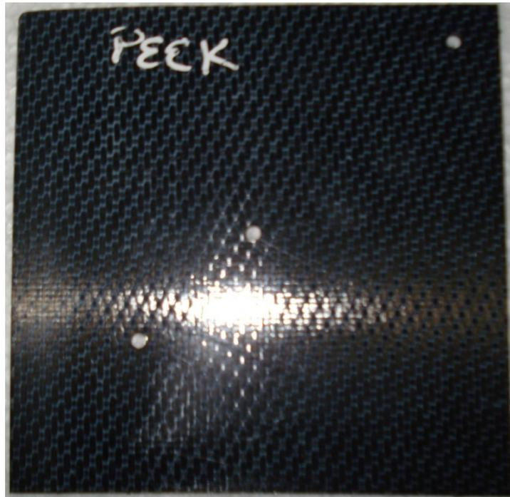
Figure 2: Sample of PEEK material with holes drilled for thermocouple fixation
