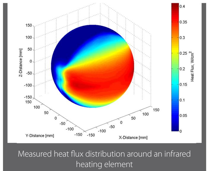
Combining the state-of-the-art IR sensing technology with state-of-the-art robotics is the true innovation of the Herschel. A specialised grip was manufactured that fixes the heat flux sensor to the wrist of a six-axis robot. Software programs were then written to position the heat flux sensor anywhere and in any position in front of heaters and heater assemblies
